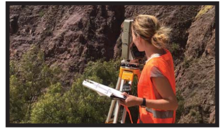
Ciara Morgan uses a total station during a trip by the Auburn University Chapter of Engineers Without Borders.
